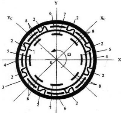
Fig. 2. Kinematic scheme of a vibrating ring gyroscope
