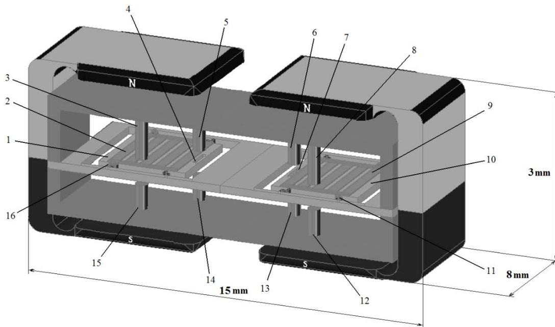
Fig. 8 Scheme of AMMG (it is not proportioned to make it more demonstrable)
