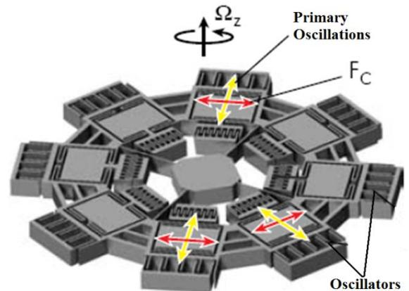
Fig. 7. The construction of distributed mass MMG
