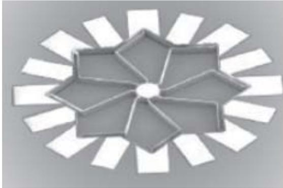
Fig. 5 SEM view of micromechanical star-shaped vibrating gyroscope
